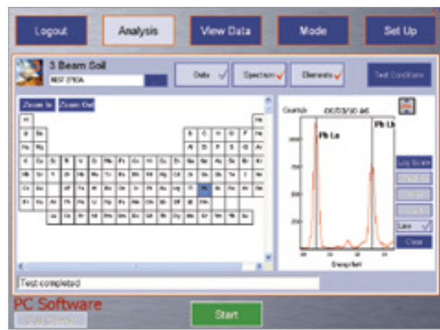
Qualitative Spectral ID on PC Software
